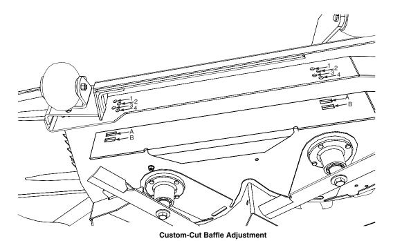
**Mounting Slot Selected Mounting Hardware Location** Slot "A" Hole 1 Hole 2 Hole 3 Hole 4 Height (inches) 3-3/4" 4-1/4" 4-3/4" 5-1/4" Slot "B" Hole 2 Hole 3 Hole 4 Height (inches) 3-1/2" 4-1/2"
